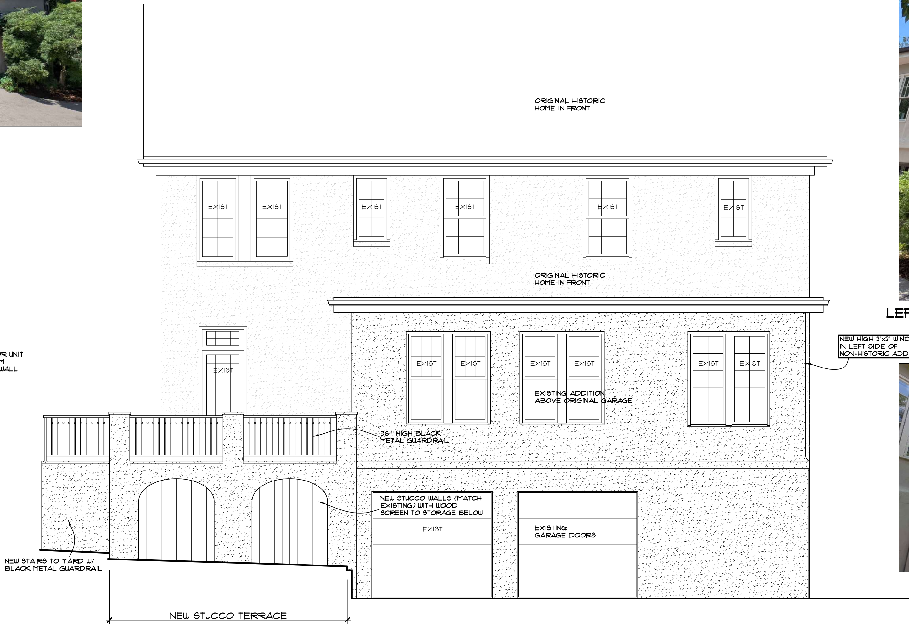
TERRACE ADDITION REAR ELEVATION SCALE: 1/4" = 1'-0"
