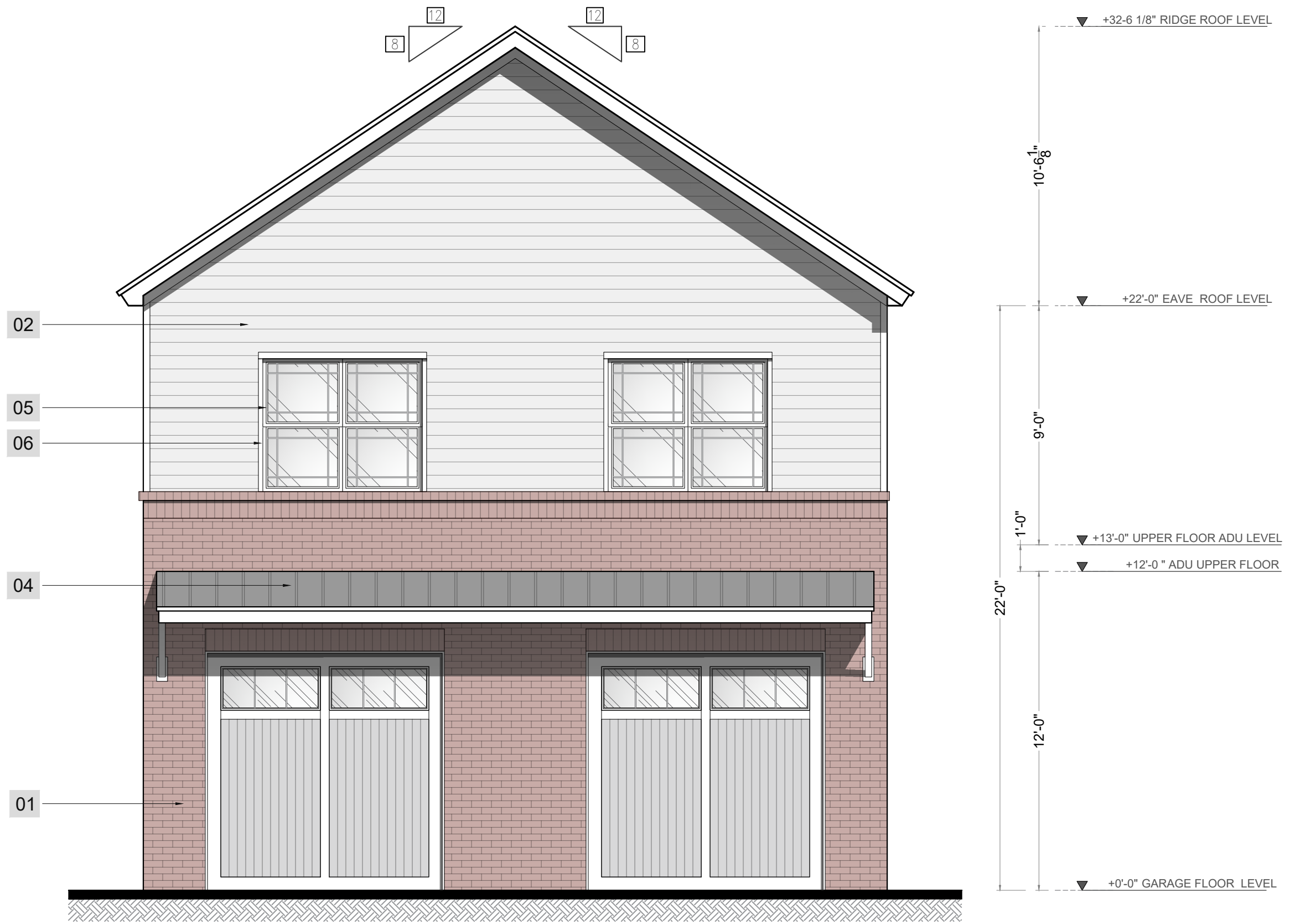
01 FRONT ELEVATION SCALE: 1/4" = 1'-0"
