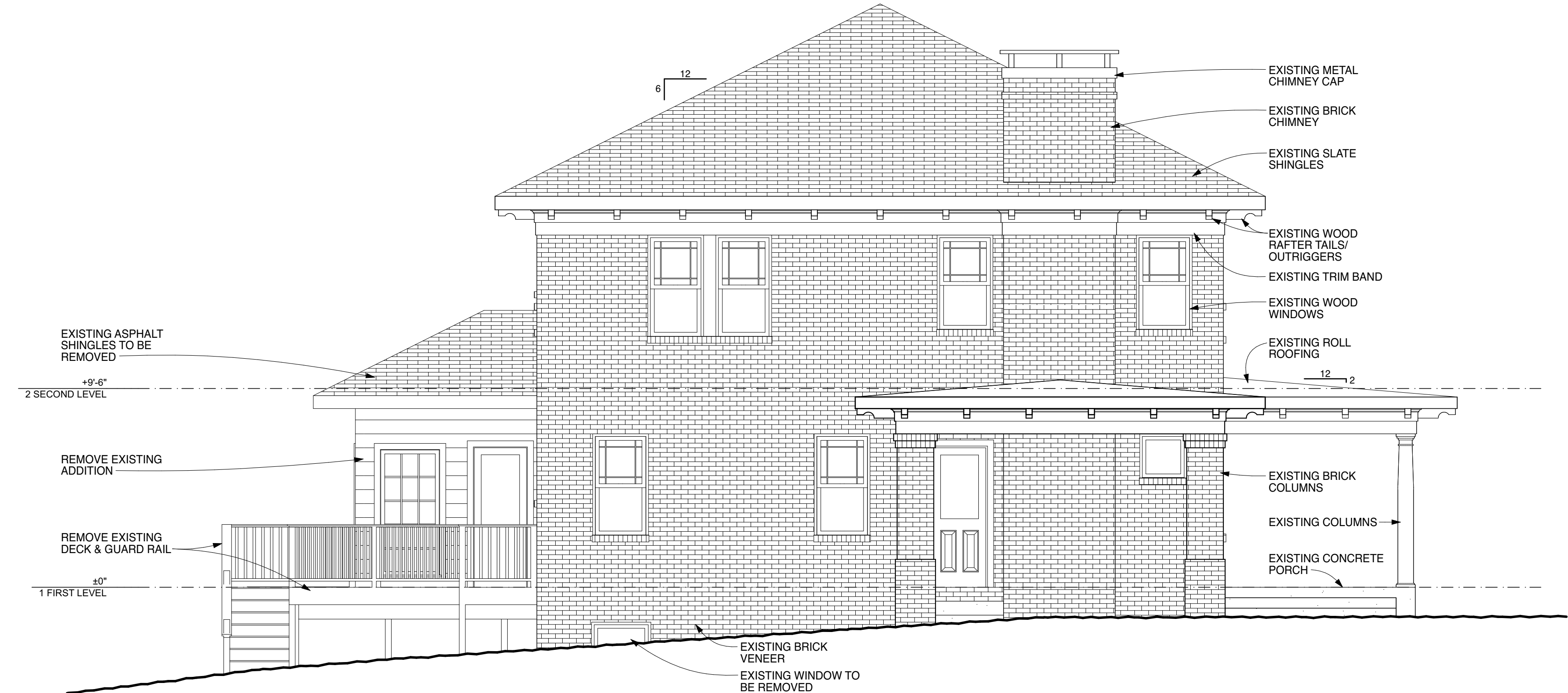
1 EXISTING LEFT ELEVATION SCALE: 1/4" = 1'-0"
