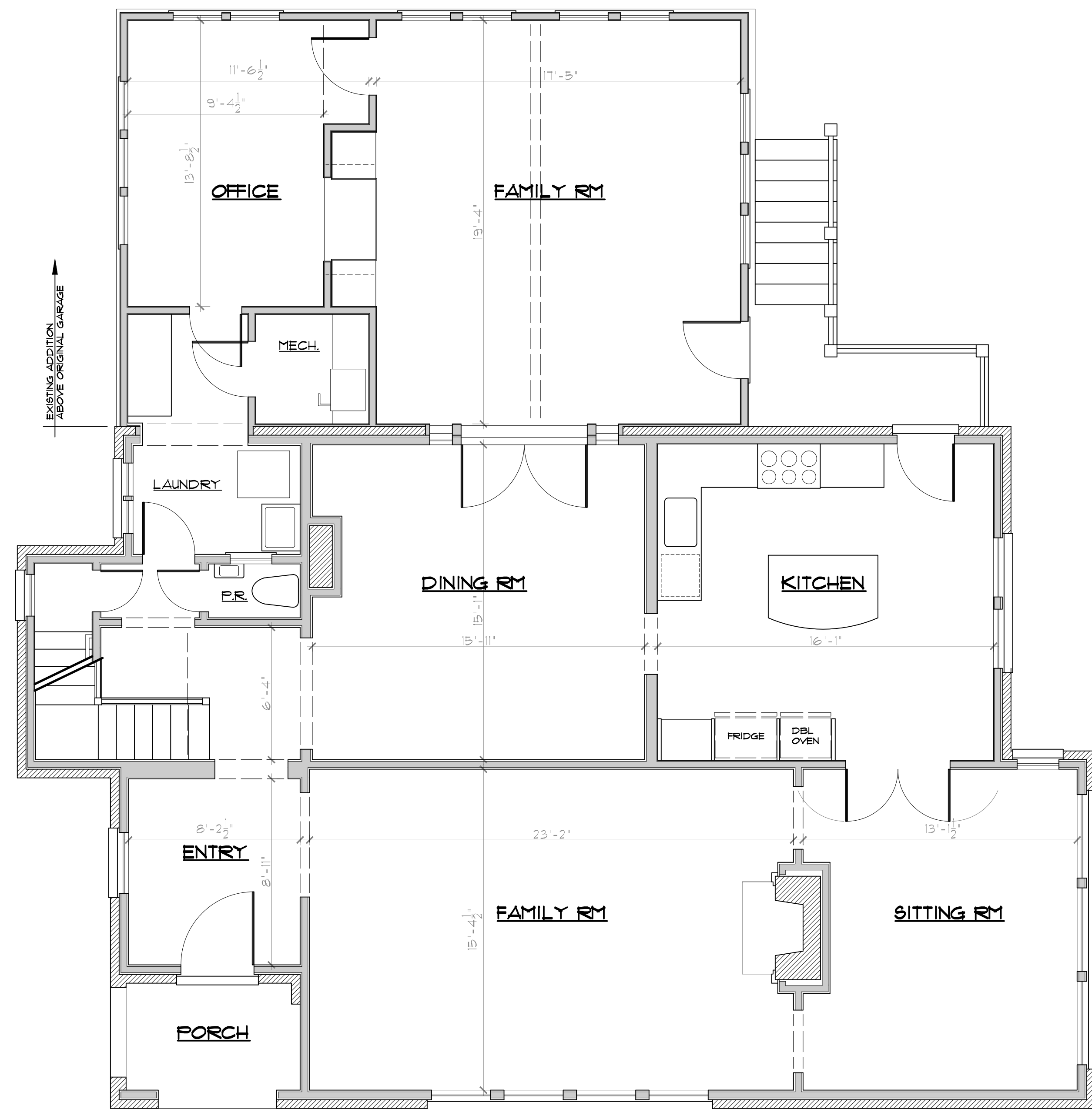
MAIN LEVEL EXISTING FLOOR PLAN SCALE: 1/4" = 1'-0"
