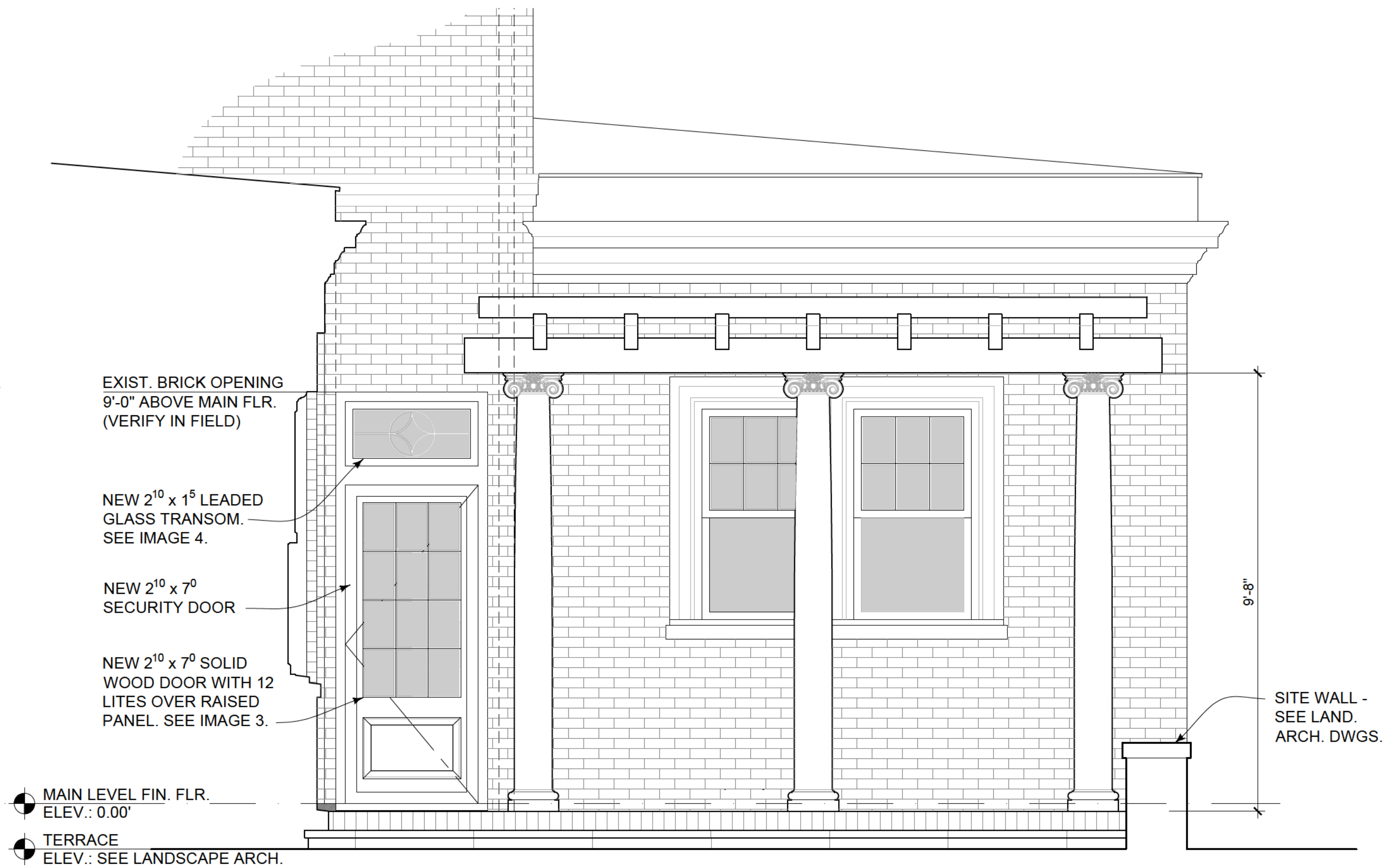
2 PARTIAL EXTERIOR ELEVATION SCALE: 1/2" = 1'-0"
