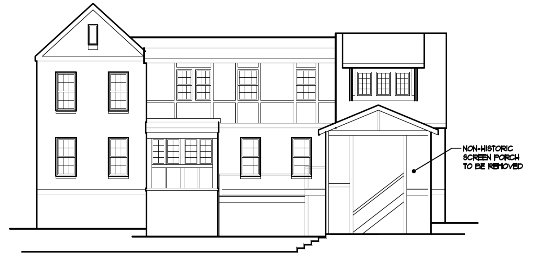
EXISTING REAR ELEVATION
