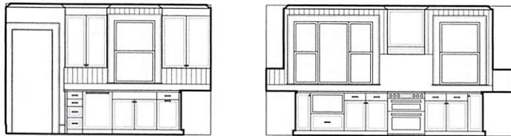
3 EXISTING KITCHEN WINDOW SASHES SCALE: 1/4" = 1'-0"
