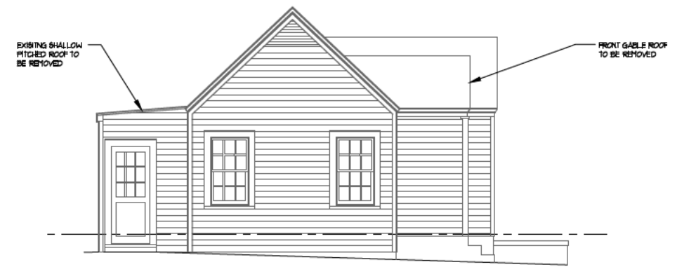
2 EXISTING NORTH ELEVATION EX1 SCALE: 1/4"=1'-0"
