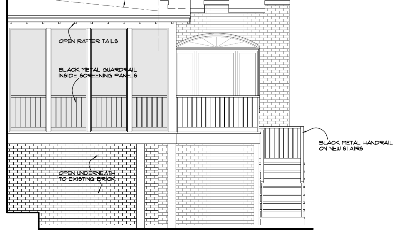
PORCH REAR ELEVATION SCALE: 1/4" = 1'-0"
