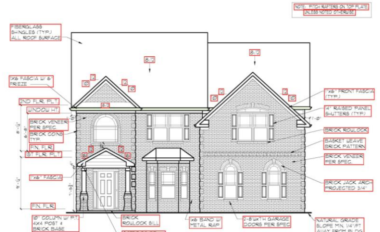
FRONT ELEVATION B1 Traditional (SCALE: 3/8"=1'-0")
