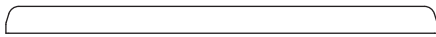
A 2 1/4" (57) width profile is available for most units to simulate a meeting rail or a multi-unit combination, such as a transom over a window or patio door.
