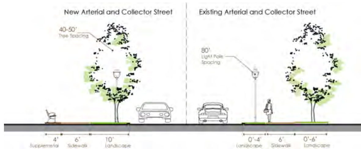
Streetscape Figure—Arterial and Collector Streets
