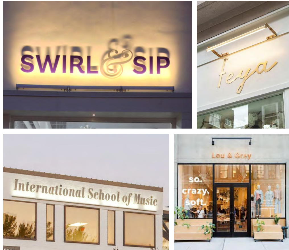
OPTION 5A: Individual Dimensional Letter Forms with LED Strip Light External Illumination
