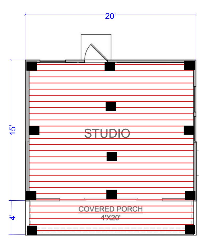
Framed 2x10 floor joist deck flooring system. 8x8 support posts.
