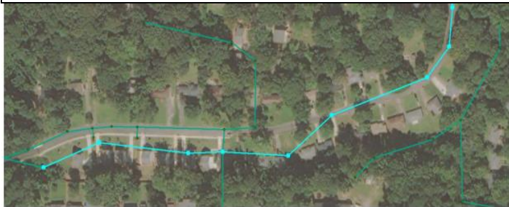
Sewer Hydraulics Profile for 15-149-s058_15-149-s057. Showing surcharging in WCTS main at 2089 Garden Circle that led to SSO from cleanout.
